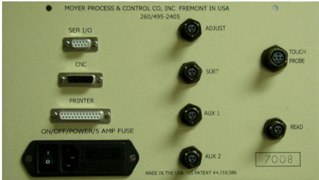
3.0.1 **PRINTER:** The 25 pin plug on the Moyer printer cable plugs into this socket. The printer cable and **MAGIC TOUCH** can be used with most Epson or IBM compatible printers. For your convenience, we keep Seiko Instruments' Inc. DPU-414 printers in stock.
