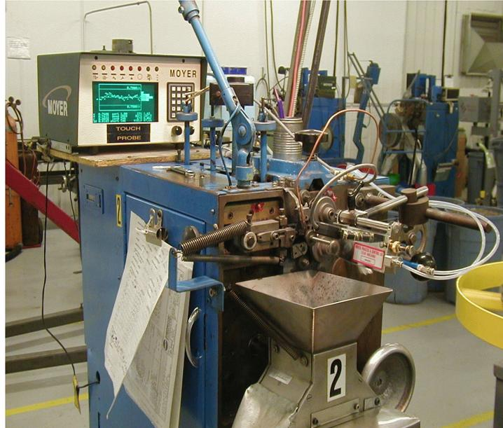
Mark the location of the holes on the coiler thru the holder base. Drill and tap holes on the coiler as marked for 1/4-20 screws. After tapping, file the coiler face to remove burrs, then mount the base & **TOUCH PROBE** mount to the coiler.
