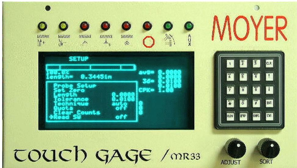
3.1.1 **Adjust Knob:** In run mode, it controls the amount of pitch adjustment. In test mode, it is used in testing the gage and probe for proper functional operation.
