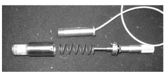
Remove the inner cylinder from the spring and replace with the new inner cylinder.
