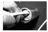
Install the micrometer so the groove for the cable in the mic end lines up with the cable coming from the inner cylinder. Use a little loctite on the screws, line up the holes and replace the screws.
