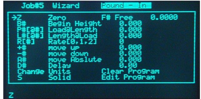
2. The first thing you want to happen is zero the loadcell, so move the cursor the **Z** and press **ENT**. Notice that a **Z** appears in the bottom left hand corner of the screen.
