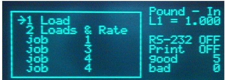
The loadcell will first **Zero**, then the ram compresses the spring to the selected height. The load will be displayed on the screen as **P1@ X.XX**.
