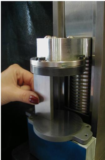
If the jo-block feels tight, loosen the cap screw 1/8 of a turn, adjust set screw, tighten cap screw.
