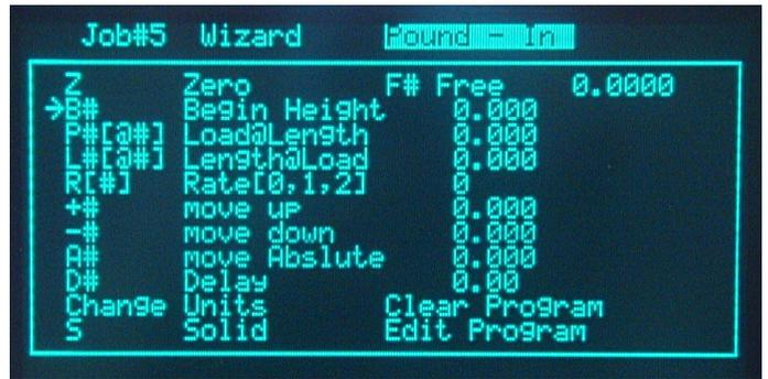
**Z** Zero Equate current loadcell force as 0.0 force to reference future readings. Used to tare or zero out the weight of the spring or to do load differential.
