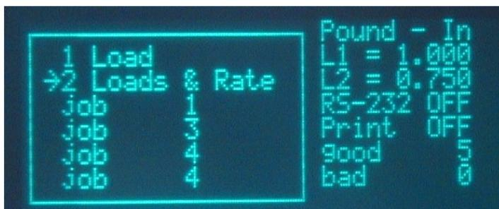
6. If using a serial data collection device, press **Y** or **(9)** at the **use RS-232 Y/N** for yes. If not, press **ENT** or **(6)** for no.
