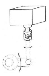
4.2.4.1b **Dual Coiling Point Systems:** The pitch control assembly consists of a pitch motor, a universal joint, and a threaded rod (often supplied with the coiler). Usually the pitch motor replaces the fine pitch adjustment knob. Remove the existing knob, detent, and universal. Check the pitch rod threads for cleanliness and rough spots. If necessary clean threads by using a die to ensure smooth movement.
