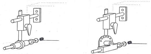
4.2.2 **Probe & Holder:** Coil a spring by hand until wire feed quits. Put the probe thru the 1" hole on the probe holder. Slide the probe forward so the collar is holding the probe at the back, close to the micrometer. Be sure you can read the micrometer. Tighten the collar around the probe using the 1/4-20 screw.
