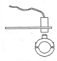
4.2.3 **Read Switch:** The read switch assembly consists of a magnet mounted on a lock collar or block and a read switch mounted on a bracket. Mount the magnet to any shaft that makes one complete revolution per spring. Mount the switch and bracket so nothing will hit it and the magnet will pass 0.030" (0.7mm) to 0.080" (2mm) from the flat on the switch. Position the read switch and magnet so the read signal will be sent after the wire quits feeding but before cut off.
