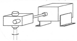
4.2.4.1a **Single Coiling Point Systems:** The pitch control assembly consists of a pitch motor, flex shaft, adaptor nut and gearbox. On some coilers, the pitch motor connects directly to the pitch rod. Remove the locking nut from the pitch rod. Check the pitch rod threads for cleanliness and rough spots. If necessary, clean threads by using a die to ensure smooth movement of the adaptor nut on the pitch rod.
