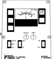
**9.2 P-P Test:** Again press the "D" button. The meter should dislay a P-P value on the meter of 95% to 105%. This P-P value represents the peak to peak drive on the mm3r1 board. It must
