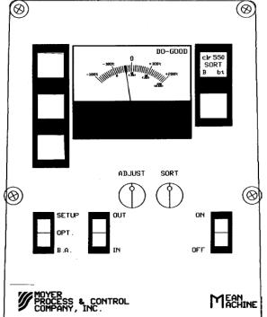
**5.2.6 SORT SHORT:** Return the micrometer to the zero position and continue turning to the short sort distance. Push the "A" (left red) button and wait until the meter stops moving. The meter should read very close to -100%. Your sort short distance is now set.
